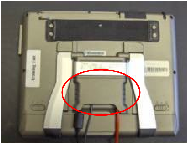
Figure 28 - Installed Cover on the Back of the Electronic Pollbook
